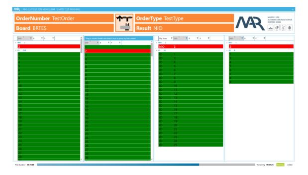
The test panel contains three main parts. Information about the current test is displayed on the top of each test panel. In the middle, the selected layout can be seen. The bottom contains the remaining time for the current test.
