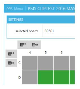
The green cells contain clips and the gray cells are empty. If some cells are not on the board, they can be excluded by clicking. Excluded cells are displayed with a white brush. Excluding cells is not required for using this test panel layout. It is only a feature used to visualize the board with its physical dimensions.
