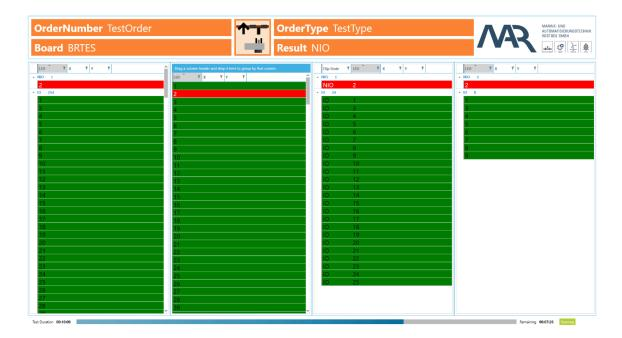
The test panel contains three main parts. Information about the current test is displayed on the top of each test panel. In the middle, the selected layout can be seen. The bottom contains the remaining time for the current test.
